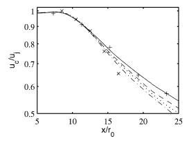
Fig. 2 Profiles of the mean centerline velocity  $u_c/u_j$  in ——, LESsf; ..., LESdsm; ---, LESre1; and --- LESre2 simulations. Measurements:  $\times$ , Stromberg et al.<sup>13</sup> (M=0.9,  $Re_D=3.6\times10^3$ ) and +, Lau et al.<sup>14</sup> (M=0.9,  $Re_D=10^6$ ). The LESdsm, LESre1, LESre2, and experimental profiles are shifted in the axial direction with respect to the LESsf profile to yield identical core lengths.
