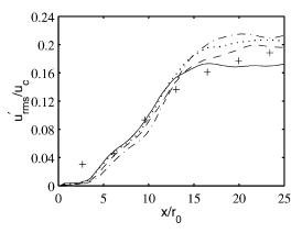
Fig. 3 Centerline profiles of the turbulence intensity  $u'_{\rm rms}/u_c$  in \_\_\_\_\_, LESsf; . . . . , LESdsm; ---, LESre1; and ---, LESre2 simulations. Measurements: +, Arakeri et al. <sup>15</sup> (M = 0.9,  $Re_D$  = 5 × 10<sup>5</sup>), shifted in the axial direction for the comparison.
