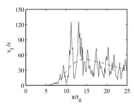
Fig. 1 Centerline profiles of the ratio  $\nu_t/\nu$  between eddy and molecular viscosities in the LESdsm simulation: ——, instantaneous and ---, time-averaged profiles.
