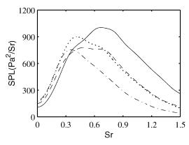
Fig. 4 Sound-pressure spectra as a function of Strouhal number  $Sr = fD/u_j$ , in linear scales, obtained in the sideline direction at  $x = 11r_0$  and  $r = 15r_0$  from ——, LESsf; . . . ., LESdsm; ---, LESre1; and ---, LESre2 simulations.
